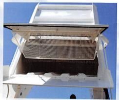
LARGEST HOPPER IN IT'S CLASS Global R4AIR includes a 5.8 cu/yd 100% Stainless Steel hopper construction, Cyclone Type Dust Separators and Swing-Down Hopper Screens are easy to Rean.
