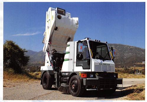
The Global R4AIR is designed to make routine maintenance easy, so your sweeper spends more time on the street and less time in the garage. Two swing-out center body panels provide unrestricted access to Fan Housing, maintenance and daily cleaning. A centralized, weather-proof systems locker fully protects electrical components from the elements while fender located Hydraulic system allows for easy maintenance, accessibility and inspection. Troubleshooting is now a breeze.
