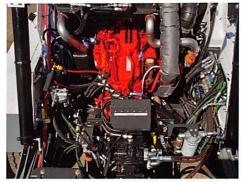
The Global R4AIR comes standard with a fuel-efficient Tier 4 Final, 6-cylinder, turbocharged 280-horsepower 6.7-liter Cummins ISB diesel engine, largest in its class, delivering outstanding performance and reliability.
