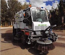
Our 47-Inch Front Articulating **Broom** is hydraulically controlled, retracts/extends, lowers/raises with additional four-way Gutterbroom tilt. All broom functions are controlled via Joystick located in the cab. The sweeping Path is extended to 139 Inches. Great for digging out curbs during heavy sweeping, and for tight cul-de-sacs and hard to reach areas.
